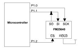
Figure 3. System Configuration without SPI port
